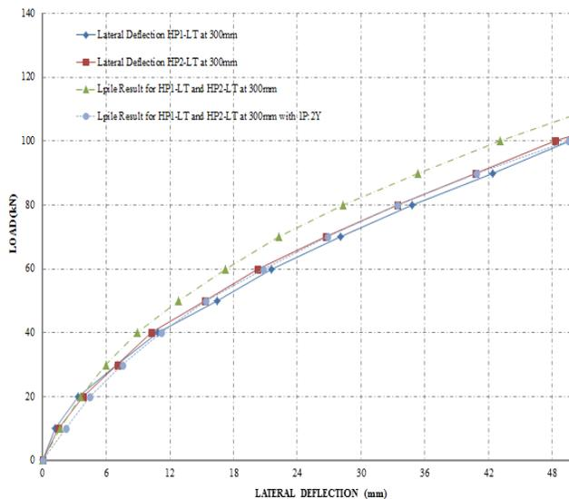
Figure 7: LPILE analysis for HP1-LT and HP2-LT
