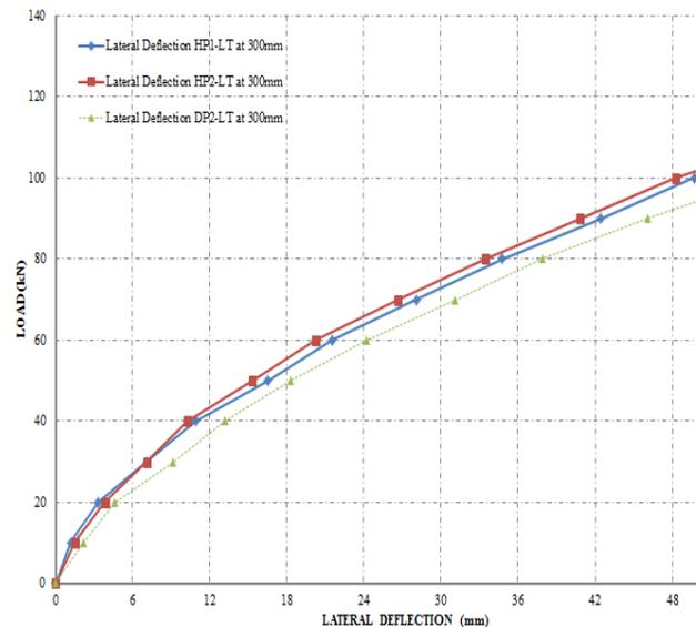
Figure 10: Comparison between long-term lateral resistance of helical piles and long-term lateral resistance of driven piles (Shorter pile group).
