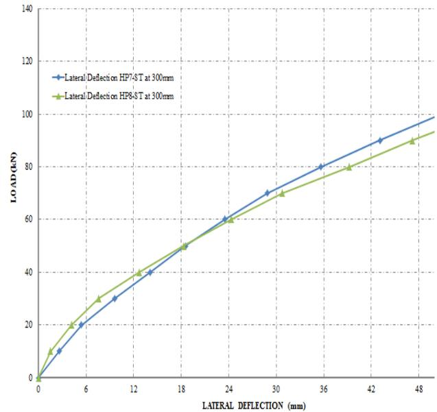
Figure 6: Lateral load-deflection curves for helical piles HP7-ST and HP8-ST
