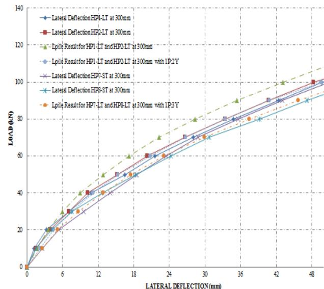
Figure 9: LPILE analysis for HP1-LT, HP2-LT, HP7-ST and HP8-ST
