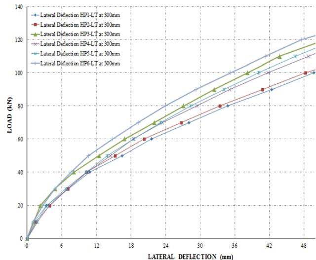
Figure 4: Lateral load-deflection curves for helical piles HP1-LT, HP2-LT, HP3-LT, HP4-LT, HP5-LT and HP6-LT
