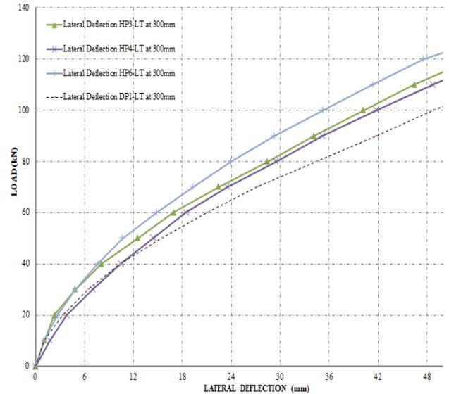
Figure 11: Comparison between long-term lateral resistance of helical piles and long-term lateral resistance of driven piles (Longer pile group).
