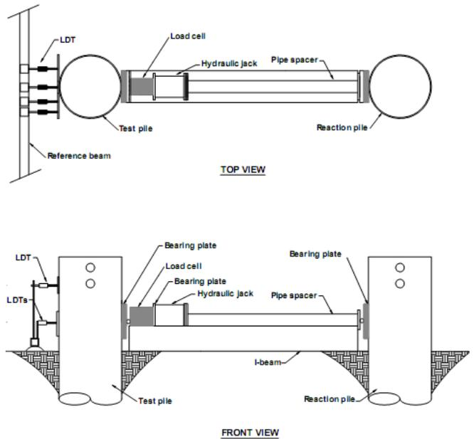
Figure 2: Typical lateral test setup
