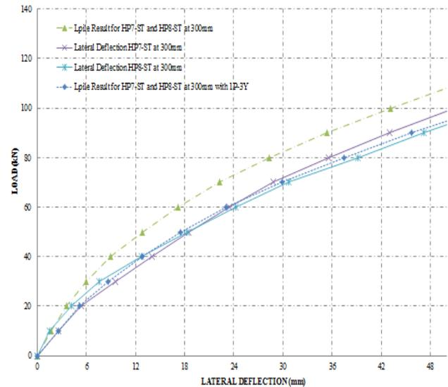
Figure 8: LPILE analysis for HP7-ST and HP8-ST
