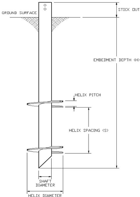
Figure 3: Helical pile configuration
