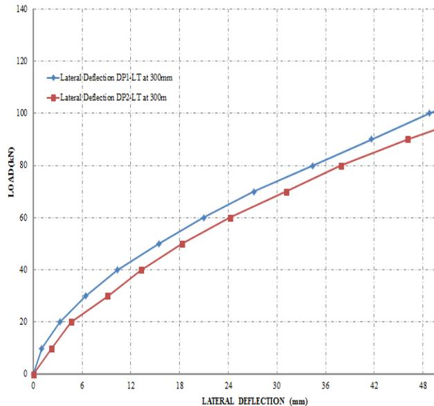
Figure 5: Lateral load-deflection curves for driven piles DP1-LT and DP2-LT
