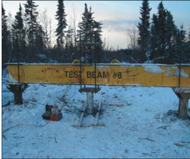
Figure 3. Typical axial tension (uplift) load test setup
